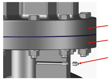
• Once the pipeline has reached its operating pressure check the gaskets and gland packing for leaks. If the gland packing is leaking tighten the gland bolting.
