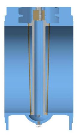
The Wedge Gate Valve is so called because of the shape of the gate and body-seating faces utilised to effect sealing.
