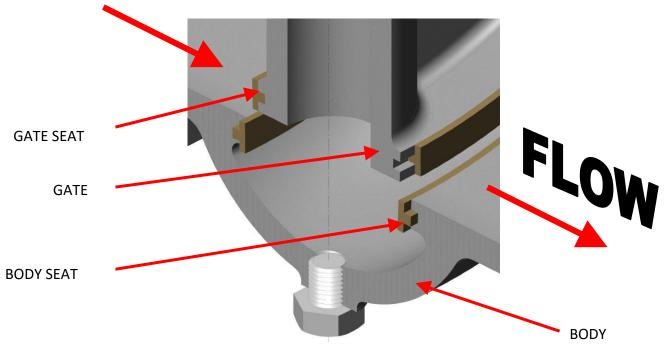
A Drain plug is fitted at the bottom of the valve body. The drain plug may be used to drain the valve 'Seat Well', in the likely event that the dirt and debris in the water has accumulated in the lower area between the sealing faces of the valve body.
