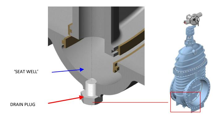
Channel Guides are fitted to the body to assist and guide the gate during the travel length of the gate in the body. These channel guides are made of Aluminium Bronze BS EN 1982 Gr CC333G (AB2).
