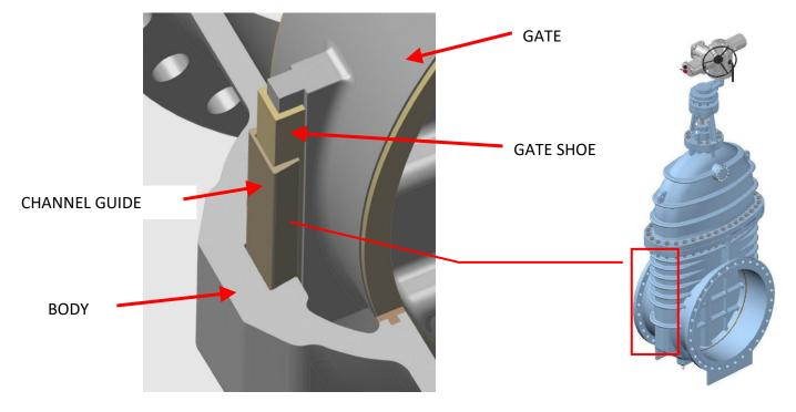
Gate shoes are fitted to the gate to assist and guide the gate during the travel length of the gate in the body
