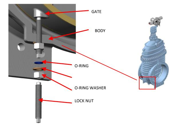
Jacking screws are fitted to the body. These are used to set the closing limit of the gate travel.
