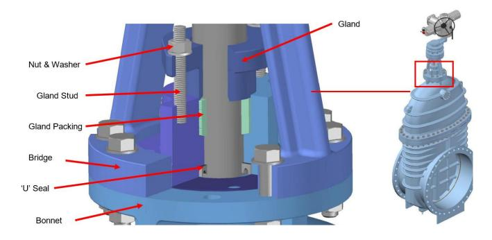
Note that during this operation a certain amount of leakage will take place however, it should notbe excessive, and should not prevent this operation being carried out.
