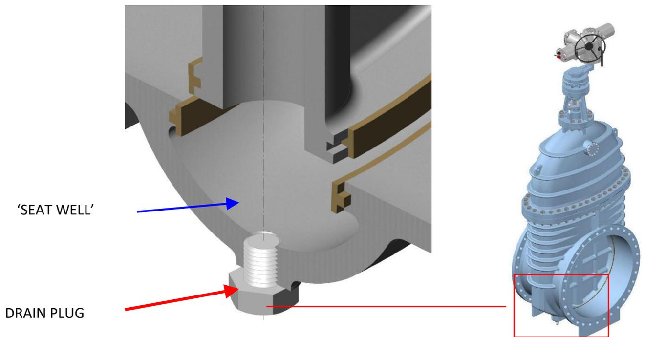
Channel Guides are fitted to the body to assist and guide the gate during the travel length of the gate in the body. These channel guides are made of Aluminium Bronze BS EN 1982 Gr CC333G (AB2).
