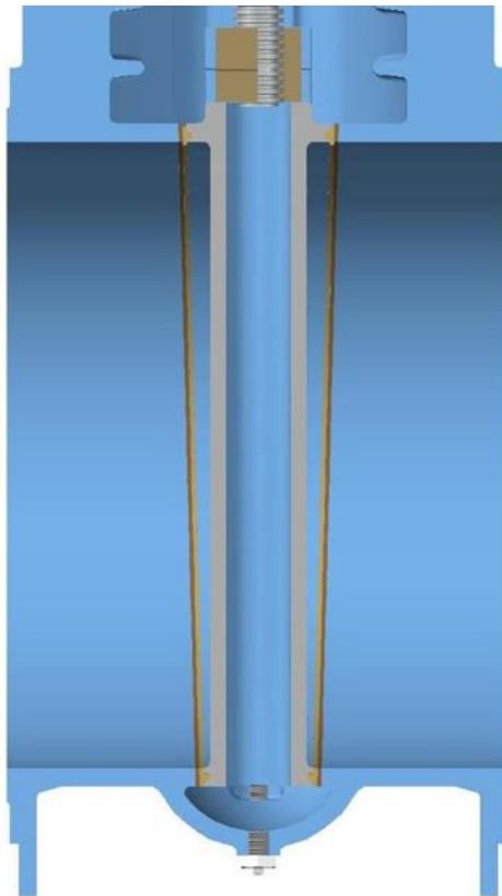
The Wedge Gate Valve is so called because of the shape of the gate and body-seating faces utilised to effect sealing.
