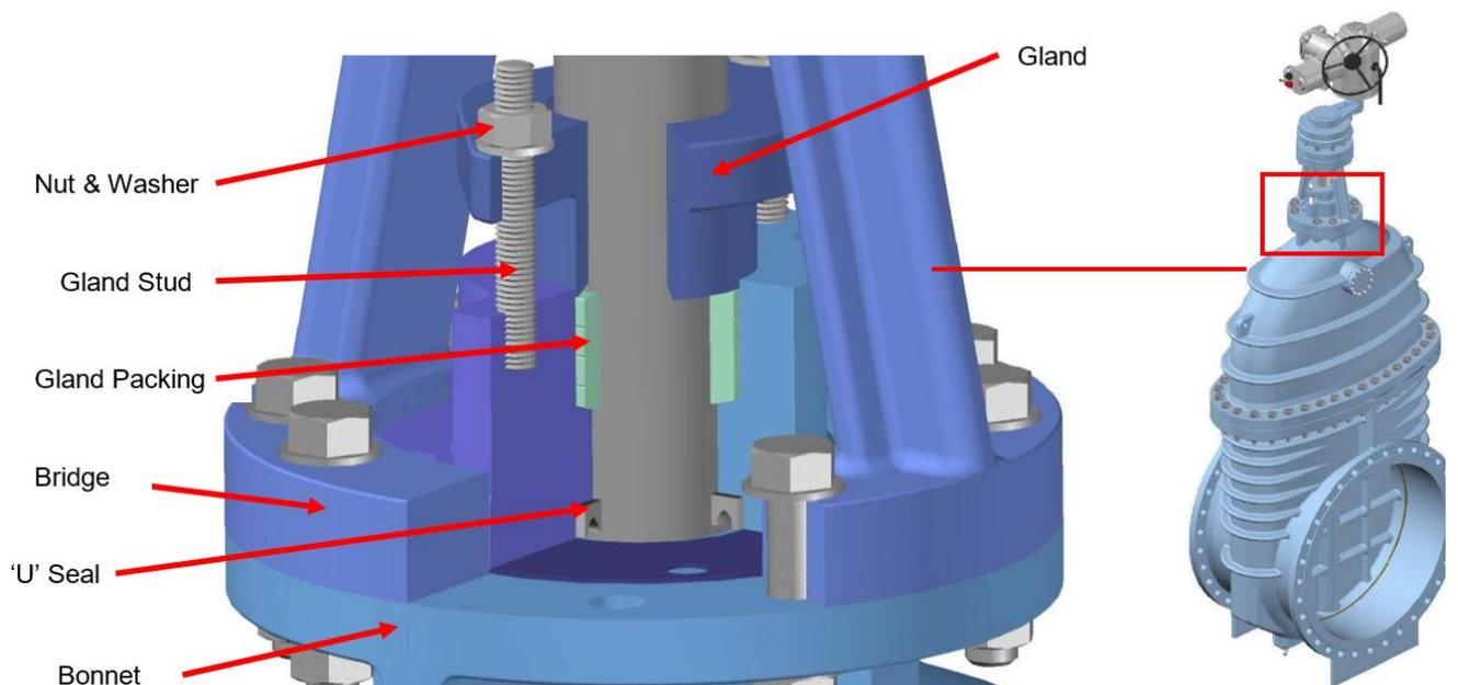
Note that during this operation a certain amount of leakage will take place however, it should not be excessive, and should not prevent this operation being carried out.
