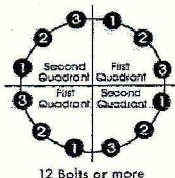
It is recommended that sufficient complete tightening circuits are carried out in sequence to ensure all bolts have attained the specified torque.
