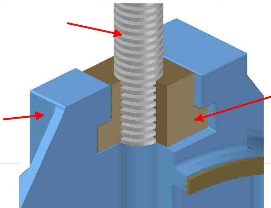
Jacking screws are fitted to the body. These are used to set the closing limit of the gate travel.
