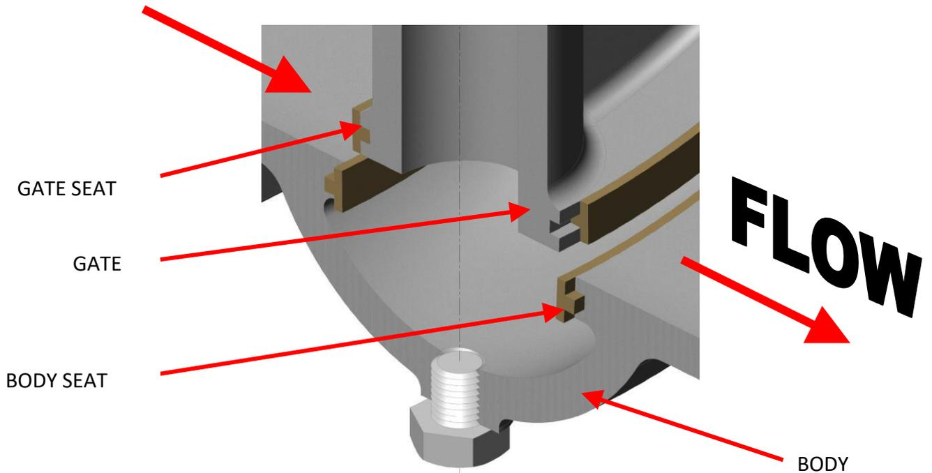
A Drain plug is fitted at the bottom of the valve body. The drain plug may be used to drain the valve 'Seat Well', in the likely event that the dirt and debris in the water has accumulated in the lower area between the sealing faces of the valve body.
