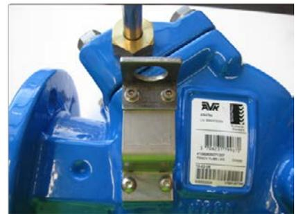
With the grub screw inserted into the proximity cam mount the proximity cam and grub assembly onto the shaft and positioning it centrally to the aperture of the proximity bracket, lightly tighten the grub screw to clamp the cam in a preliminary position.
