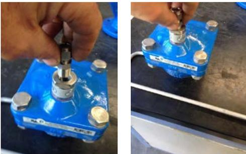
2. Screw in male connector by hand until firm (Use a sealant or thread tape to seal).
