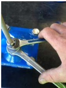
5. Insert stainless steel tube ensuring it bottoms out on male connector, use appropriate size spanner to tighten ferule nut while insuring the male connector body is held in position as not to turn.
