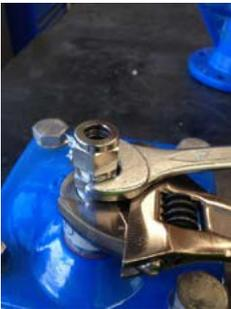
4. Use appropriate sized spanner to tighten the male connector body.
