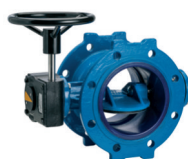
Series 756 Double Eccentric butterfly valve, bare shaft Ductile iron body and disc with epoxy coating Integral Body Seat Stainless steel shaft with self-lubricating bearings Short face-to-face Designed to EN593 Face- to-face according to EN558 T2
