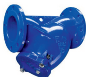
Series 910/21-001 Y-strainer with screen, plug and fasteners in SS-304 Ductile iron EPDM high temperature Blue epoxy RAL 5017 250 µm
