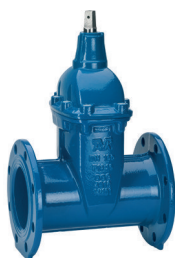
Series 43/60 Flanged gate valve Face-to-face to SANS/ EPDM rubber Ductile iron Options: • Flange drilling to Pn16 Tab. D or Bs10 D • Clockwise to open or clockwise to close • DN50-600
