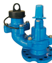
Series 29/387-004 Underground fire hydrant, London round outlet, CTO, red stemcap, SABS Approved, PN10/16, design to BS750 Ductile iron EPDM seals, WRAS approved Epoxy coated according to WIS 4-52-01 class B Clockwise to Close, Stem Cap/White Insert Locally manufactured
