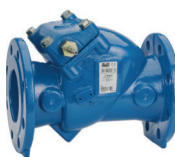
Series 41/60 Swing check valve Face-to-face to EN558-48 SANS664 coating Ductile iron DN50-300 Drinking Water
