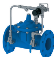
Series 869/200X-001 Reduced bore control valve, pressure reducing, SS-304/DI trim, PN10/16 Face-to-face dimension according to EN 558, basic series 1 Ductile iron EPDM rubber, WRAS approved Blue epoxy RAL 5017 300 µm
