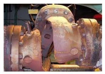
Water Hammer; Typically caused when a body of water hits an obstacle; for example a valve which is closed too quickly, will send a shock wave along the pipe with the potential to destroy both the pipe and equipment.
