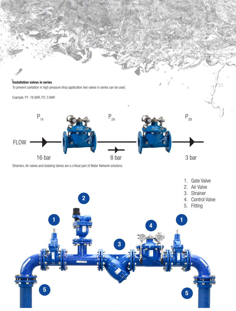
Above image is an example, always use 5 x pipe diameter of straight pipe either side of control valve as industry reccomendation.
