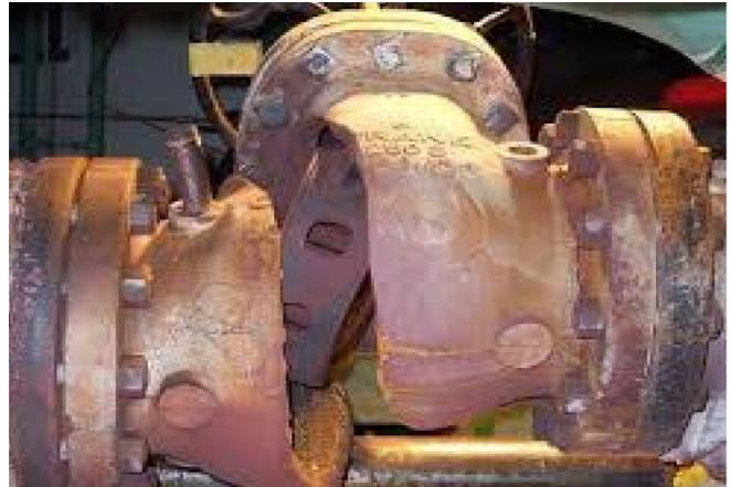
Water Hammer; Typically caused when a body of water hits an obstacle; for example a valve which is closed too quickly, will send a shock wave along the pipe with the potential to destroy both the pipe and equipment.
