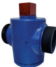
Series 6127/13-001 Cementation High pressure Plug/Cock Valve, 2" bore (55 mm), 2" x 2 1/2" female/female BSP, nitrile seal, nylon packing Steel
