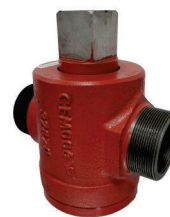
Series 6127/16-001 Cementation High pressure Plug/Cock Valve, 2" bore (55mm), 2" x 2 1/2" female/male BSP, nitrile seal, nylon packing
