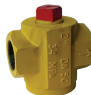
Series 6127/08-001 Cementation High pressure Plug/Cock Valve, 2" bore (46 mm), 2" female BSP, nitrile seal, nylon packing Steel
