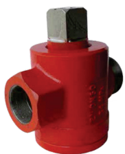
Series 6127/13-001 Cementation High pressure Plug/Cock Valve, 2" bore (55 mm), 2" x 2 1/2" female/female BSP, nitrile seal, nylon packing Steel
