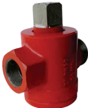
Series 6127/07-001 Cementation High pressure Plug/Cock Valve, 2" bore (55 mm), 2" x 2 1/2" female/male BSP, nitrile seal, nylon packing Steel
