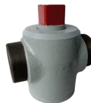
Series 6127/12-001 Cementation High pressure Plug/Cock Valve, 3" bore (77 mm), 3" thread female/male BSP, nitrile seal, nylon packing Steel Also available in 80mm bore (blue colour)
