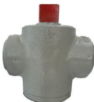
Series 6127/11-001 Cementation High pressure Plug/Cock Valve, 2 1/2" bore (63.5 mm), 3" female BSP, nitrile seal, nylon packing Steel
