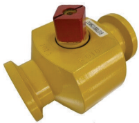
Series 6127/06-001 Cementation High pressure Plug/Cock Valve, 1 1/2" bore (40 mm), 2" hub for hub clam, copper seal, nylon packing Steel
