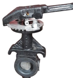
Series 6144/02-001 ASTM A216 WCB AVK Butterfly Valve, Wafer Rubberlined BFV Fixed Liner PN25 DN50 - DN150 Lever Operated DN200-DN600: Gearbox Operated
