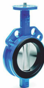
Series 820 • Body Construction B1 Wafer DN 32-600 B3 Lug DN 32-400 B4 U-section DN 450-900 • Face to face dimension according to ISO 5752/20, EN 558-1/20 • Top flange according to EN ISO 5211 • Max, working pressure 16 bar (DN32-150) 10 bar (DN200-300) 6 bar (DN350-900) • Flange connection PN10, PN16, ANSI ci. 150 AS 2129 table D + E and others
