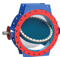
Series 6137 Boving Double Eccentric Butterfly Valve Soft seal S.G. Iron body and disc Bare shaft PN10-PN40 Options: • Locking Device • Coating above 400µ FBE • Coating to DN500 • Seat and Clamp Ring • 316 SS A4 bolts • Drinking, Waste and cooling water
